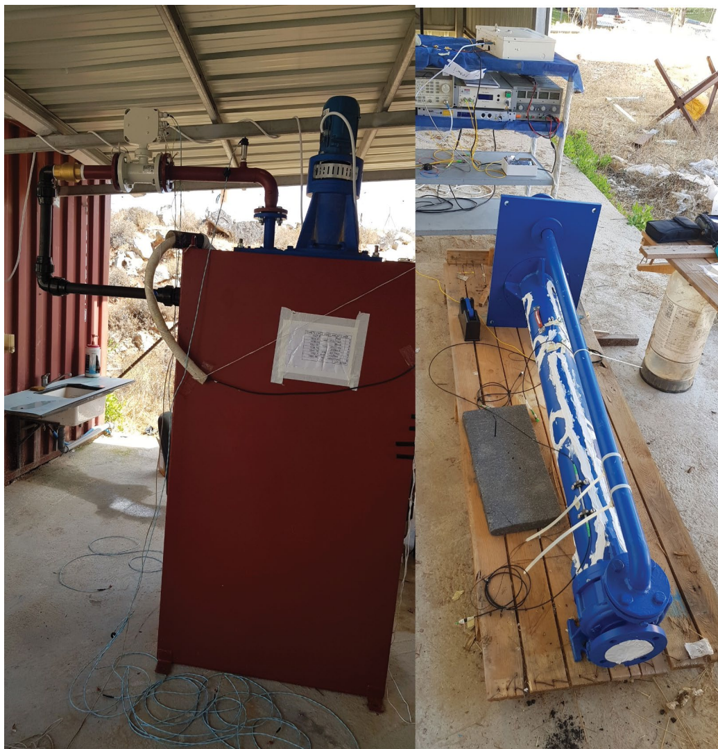
Figure 1: Left: Semi-submerged vertical pumping system consists of a 1.5 m submerged pump in a water tank with a flow-controlled water circulating pipe. Right: Sensor installation.
